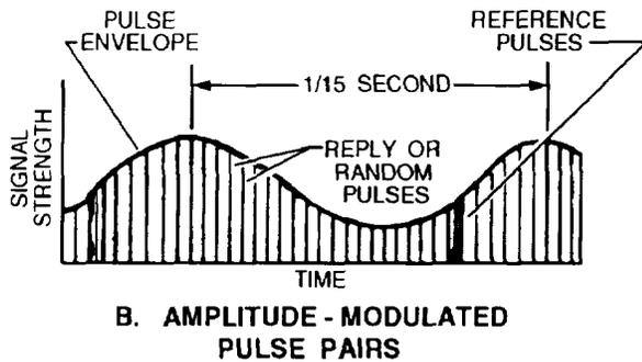
**Figure 2-5.—TACAN radiation pattern: A. cardioid pattern; B. Amplitude-modulated pulse pairs.**
