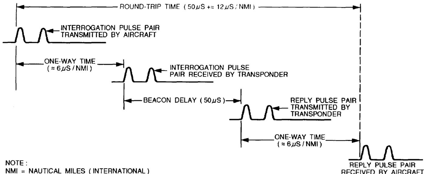
Figure 2-2.—Distance measuring round-trip travel time.
